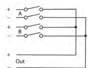
DigESwitch Differential Mux-(one channel shown)
